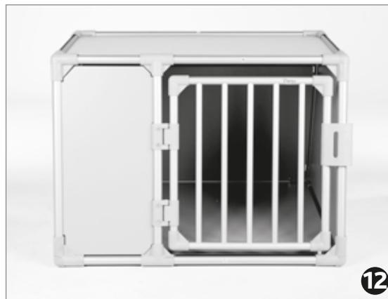
Fit the door into the hinges and screw the pins tight. The door is fitted correctly if it can be opened by lightly pressing on the fastener at the front. This is a security feature to prevent undesired opening (e.g. through the dog from the inside) and rattling. If the door is difficult to open or to close, this indicates that the screws have not been tightened enough or one of the panels is not quite straight.
