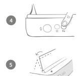
Start to increase the motion of the lid by pressing the Training Function (**Fn**) button once again. The lid will close a small amount and the light will flash orange twice.
