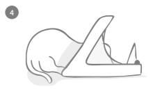
When your pet eats from the bowl and has been learnt, the light will stop flashing and remain on. When your pet moves away from the feeder the lid will close and the green light will turn off. Their microchip number is now stored permanently in memory, even when the batteries are removed.
