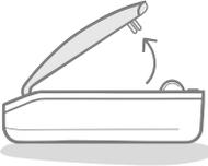
Hold one of the lid guides near the rear and pull it upwards until you are able to unhook the front section. You will need to pull it hard! Then do the same to remove the second lid guide.
