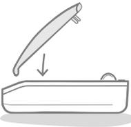
To replace the lid guides repeat the process but in reverse. Make sure that you hook them in at the front first and then attach the back.
